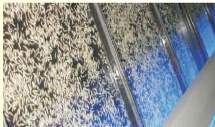
takes full control on the defect size of the rice, length and width. Every single particle that doesn't fit with the programmable one is removed. The Sortex machine ensures that the discolored grains of rice like yellow or black do not get mixed with the final product and the packed rice is in fact only white in color.
